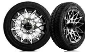
12" Athena Gloss Black and Machined Alloy Wheel With 205/40-12 Steel-belted Radial Tires
